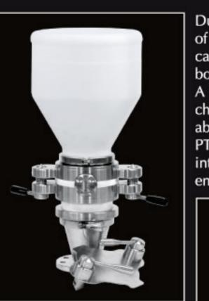
Due to the unique properties of the PTFE seal the valve can be used for charging both powders and liquids. A full range of customised charge drums are also available in stainless steel, PP, PTFE or HC22 complete with integrated spray nozzles to ensure a complete charge.
